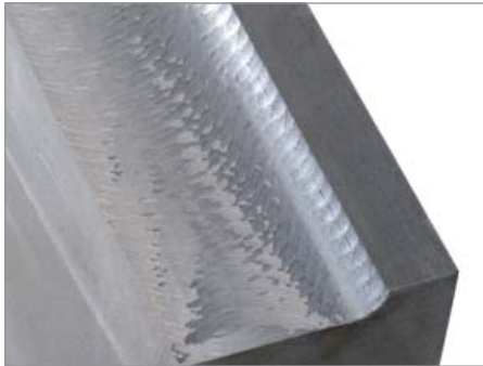
Heavy cutting without ACC
