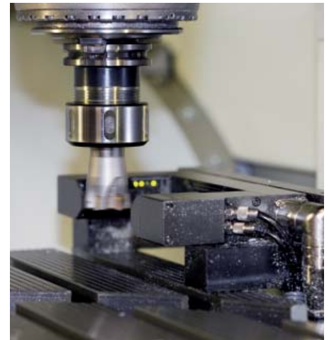
Inspection of individual tooth shape
